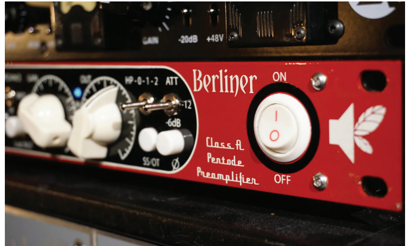
The Sonic Farm Berliner is a dual-channel hybrid microphone preamplifier that is very loosely based on the Telefunken V76.
