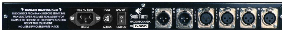
Fig. 2: Latching, balanced XLRs for mic inputs and line I/O grace Berliner's rear panel.
